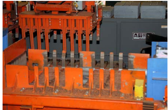
Robot Tooling and Stacker Side Plates fit neatly together preventing brick from turning over.
