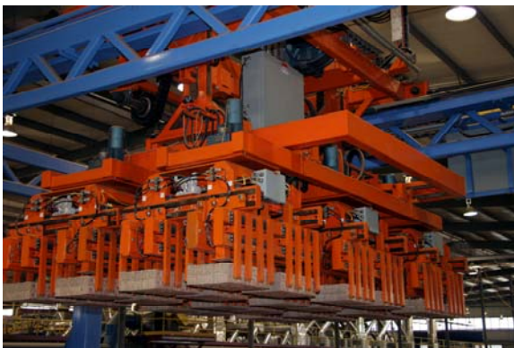
Special six gripper deheading head that spreads and rotates
