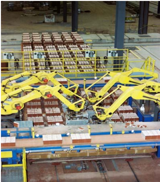
Four Fanuc 410 iWW Robots unload brick from the kiln car.
