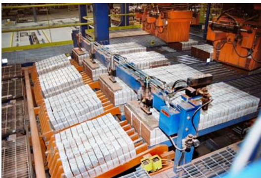
The marshalling system features a unique counting/split system that allows for easy counting of all brick sizes, even the split pavers.
